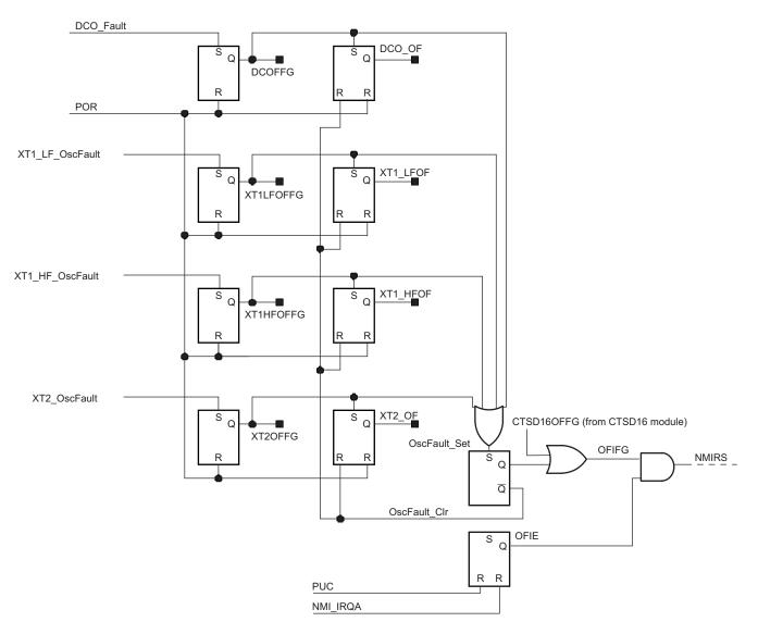
Figure 1-4. Oscillator Fault Logic
