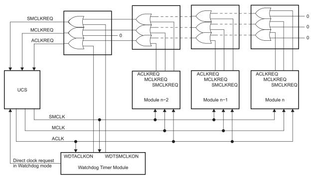
Figure 1-3. Module Request Clock System
