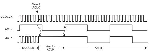
Figure 1-5. Switch MCLK from DCOCLK to XT1CLK
