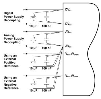
Figure 1-12. ADC12 A Grounding and Noise Considerations
