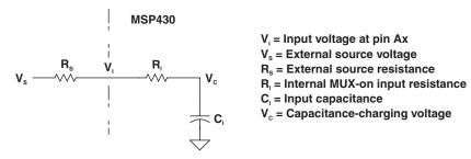
Figure 1-6. Analog Input Equivalent Circuit
