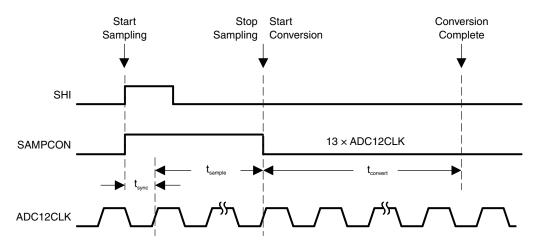
Figure 1-5. Pulse Sample Mode
