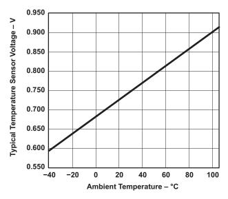
Figure 1-11. Typical Temperature Sensor Transfer Function
