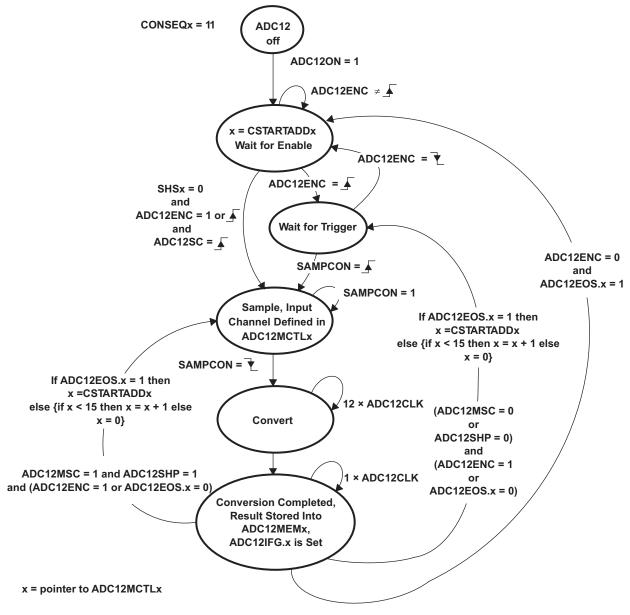
Figure 1-10. Repeat-Sequence-of-Channels Mode
