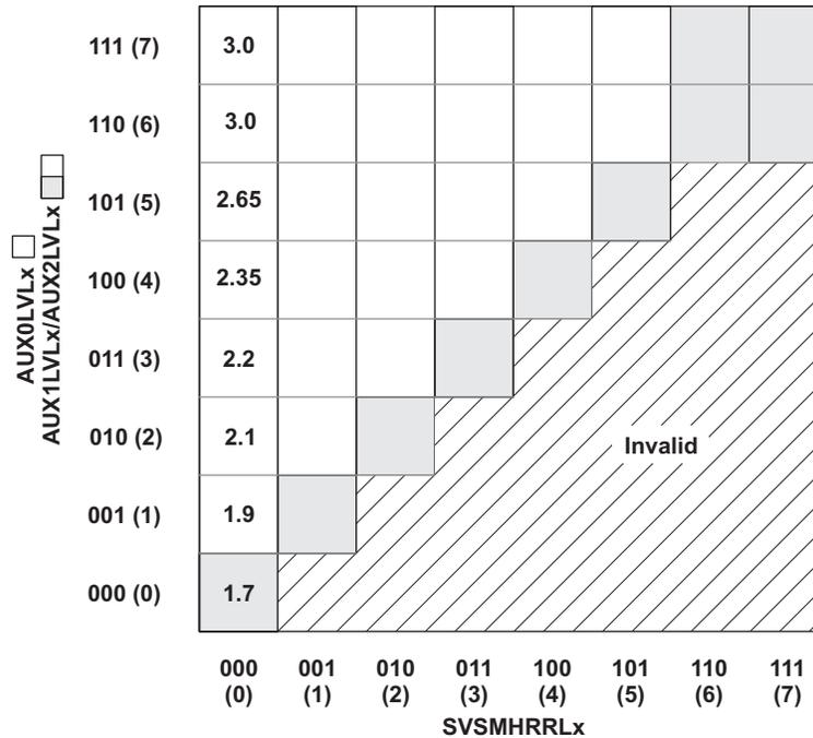
Figure 1-4. Available AUXxLVL Settings vs SVM<sub>H</sub> Settings
