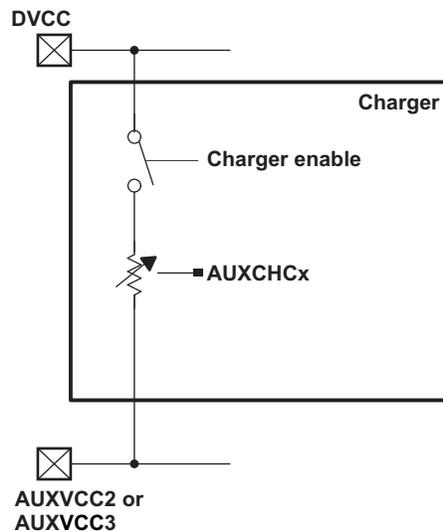
Figure 1-8. Charger Block Diagram
