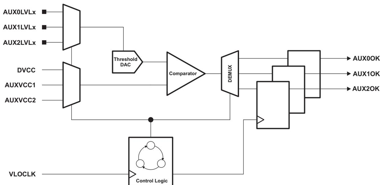
**Figure 1-5. Auxiliary Supply Monitor Block Diagram**
