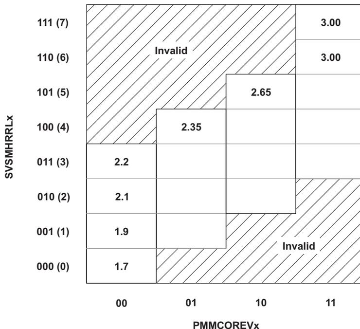
**Figure 1-3. Available SVM<sub>H</sub> Settings vs V<sub>CORE</sub> Settings**
