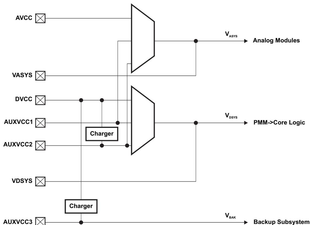
**Figure 1-1. Auxiliary Supply Switch Overview**
