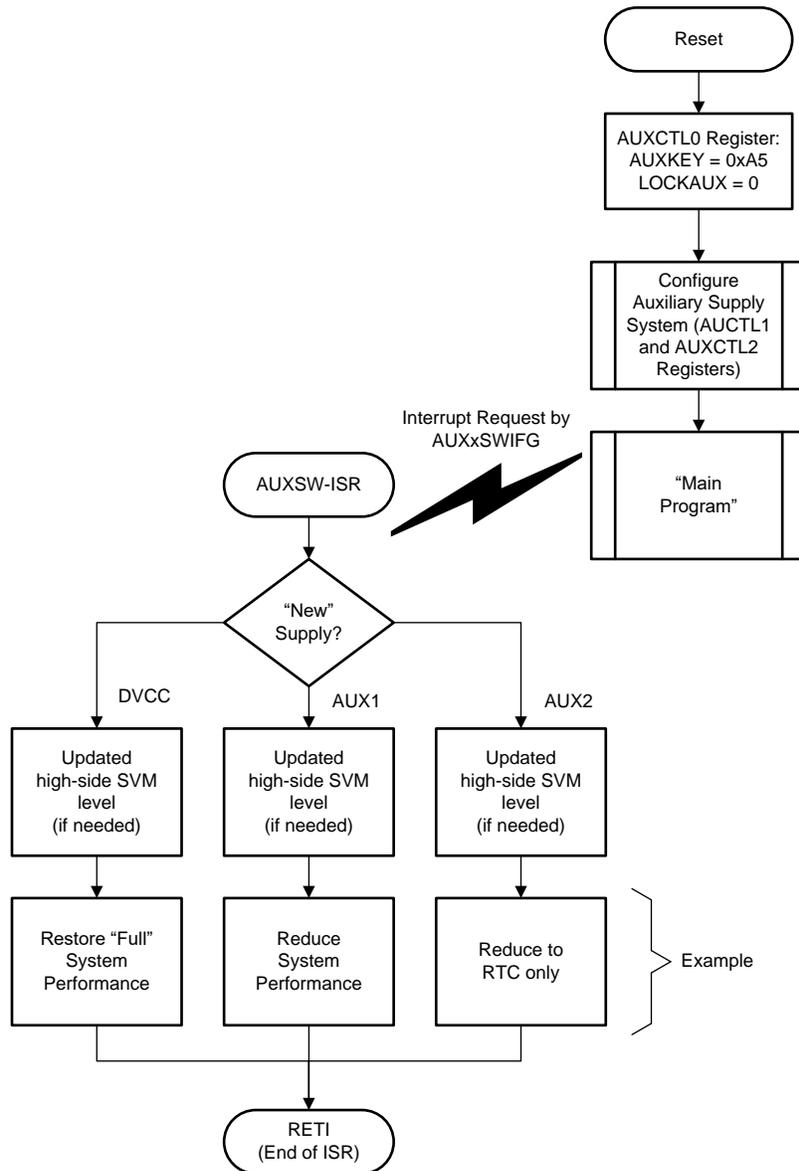
NOTE: Configuration of the auxiliary supply system is required after wakeup from LPMx.5. None of the AUX registers are retained during LPMx.5.
