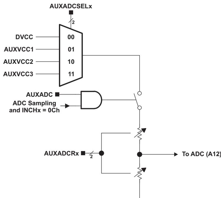
**Figure 1-7. AUX Connection to ADC**
