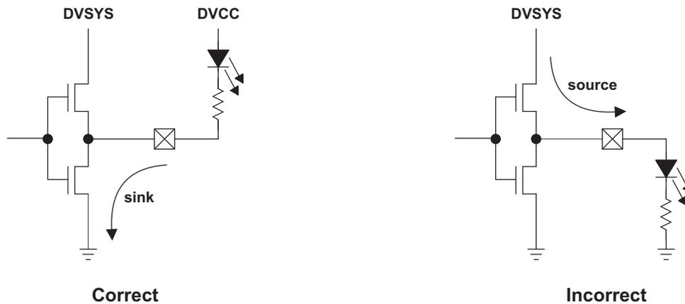
**Figure 1-6. I/Os Powered by Auxiliary Supplies**
