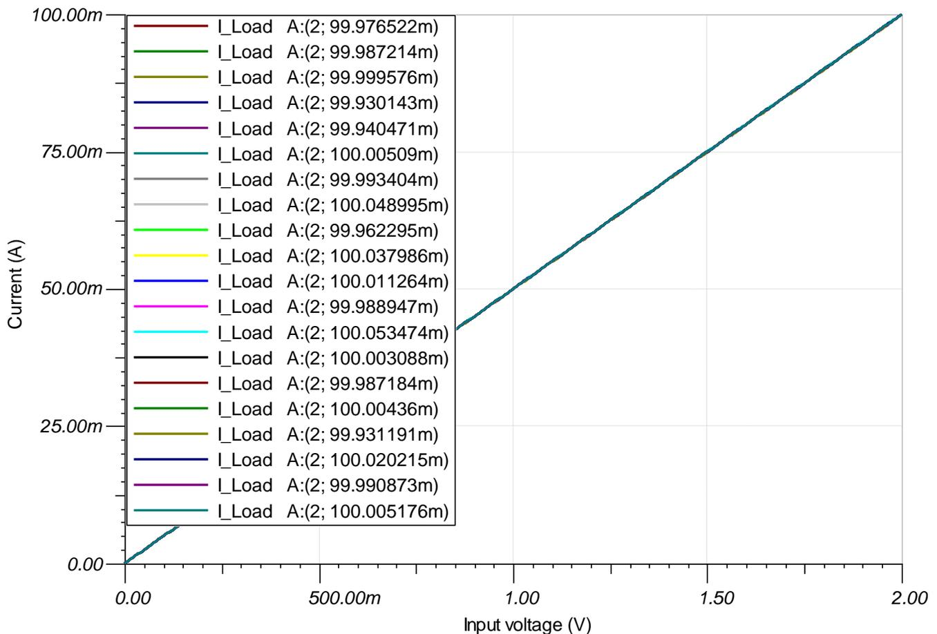
**Figure 5. TINA-TI™ - I<sub>LOAD</sub> Monte-Carlo DC Transfer Function**
