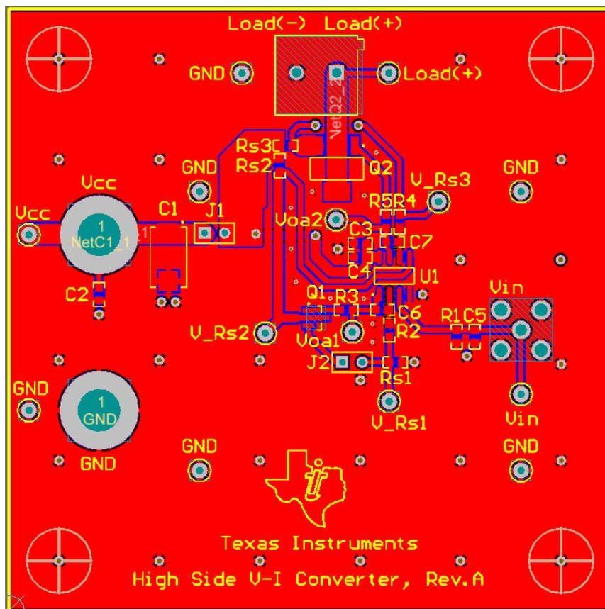
Figure 8. PCB Layout
