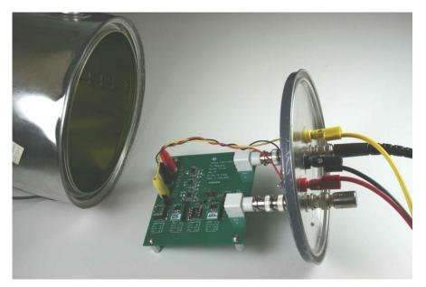
Figure 20: Shielded environment used to measure noise
