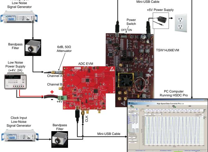
Figure 2. EVM Test Setup
