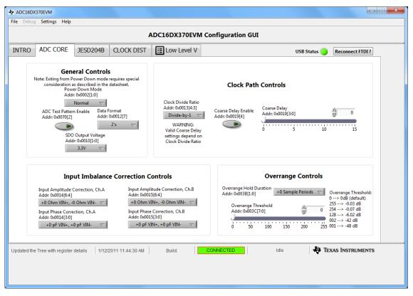
Figure 5. Configuration GUI ADC Core Tab
