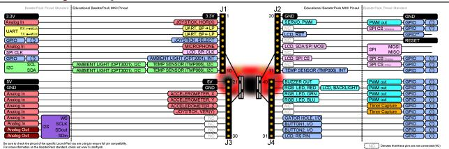
Figure 2-2. BoosterPack Plug-in Module Pinout
