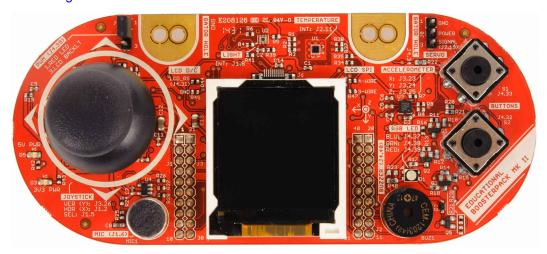
Figure 1-1. BOOSTXL-EDUMKII BoosterPack Plug-in Module
