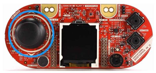
Figure 3-2. 2-Axis Analog Joystick With Digital Input
