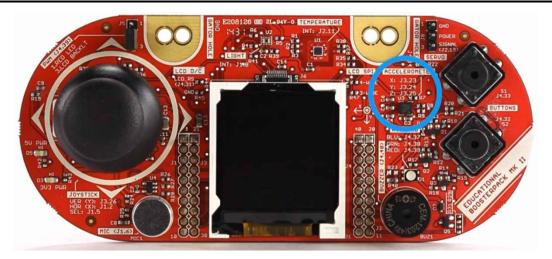
Figure 3-1. 3-Axis Analog Accelerometer
