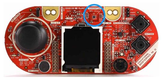
Figure 3-4. TMP006 Infrared Contactless Temperature Sensor
