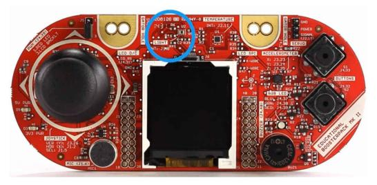
Figure 3-3. OPT3001 Ambient Light Sensor
