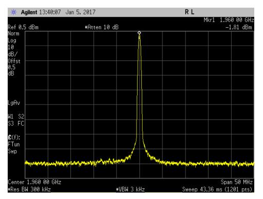
Figure 3. DAC Output Spectrum
