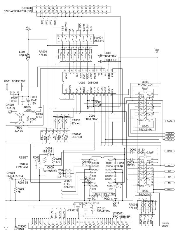
Figure 2-1. DEM-DAI1808 Digital Section (Digital Audio Interface)
