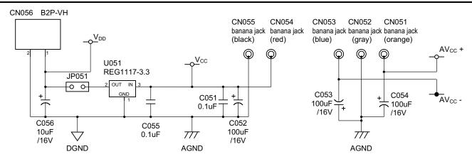
Figure 2-2. DEM-DAI1808 Regulator and Connector
