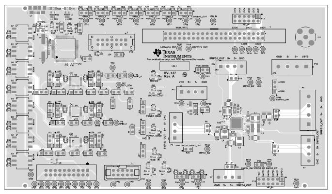
Figure 7. Composite - Top View
