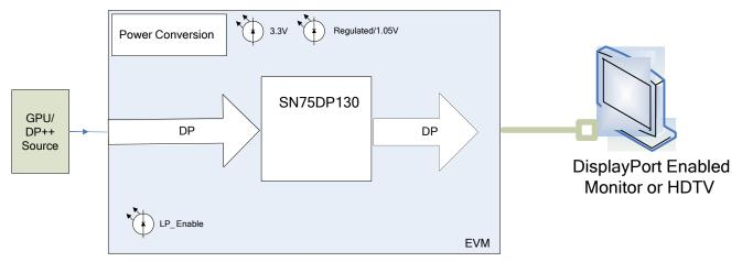
Figure 1. SN75DP130 EVM Block Diagram
