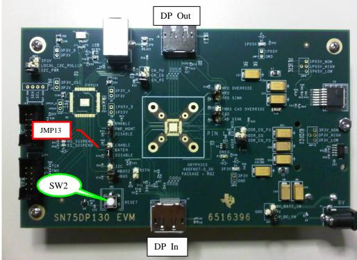
Figure 2. SN75DP130 EVM Switch and Jumper Location (Top)
