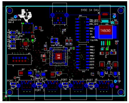
Note the EVM dimensions of  $3" \times 4"$  accommodates various lab test components, actual production implementations can be much smaller. Also, the TUSB8040A1EVM is laid out to accept either a TUSB8040A1 unit or a socket. This socket functionality would not need to be duplicated on a production implementation.
