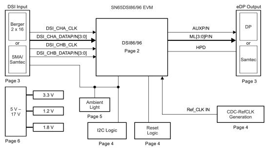
Figure 3. SN65DSIX6 EVM Block Diagram
