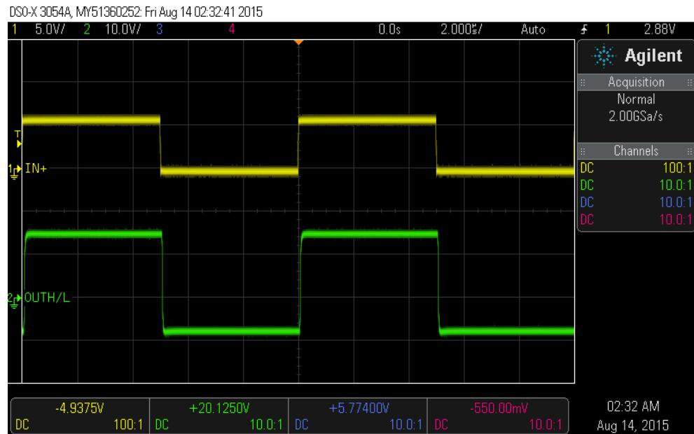
**Figure 5.** ISO5852S EVM Input and Output With Bipolar Output Supply ( $V_{CC2} = 15 V$ ,  $V_{EE2} = -8 V$ )
