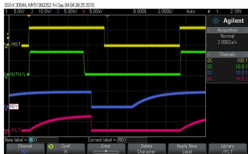
**Figure 7. ISO5852S EVM OUTH/L, RDY,  $\overline{FLT}$ , and  $\overline{RST}$  With Unipolar Output Supply**
