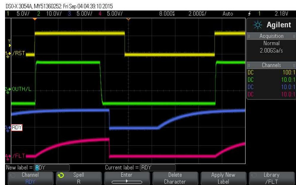
**Figure 9. ISO5852S EVM OUTH/L, RDY, FLT, and RST With Bipolar Output Supply**
