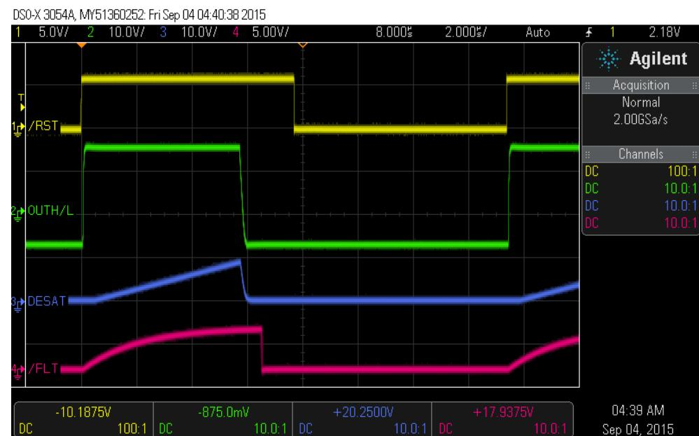
**Figure 8. ISO5852S EVM OUTH/L, DESAT,  $\overline{FLT}$ , and  $\overline{RST}$  With Bipolar Output Supply**
