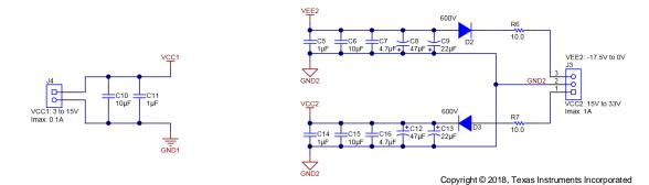
Figure 2. UCC5390ECDWVEVM Power Supply Schematic
