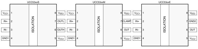
Figure 1. UCC53x0 Pin Configurations
