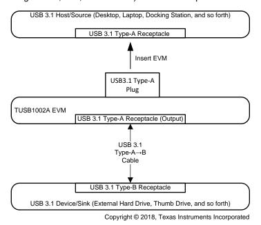
Figure 1. TUSB1002A Functional System Level Block Diagram
