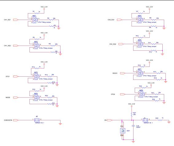
Figure 4. TUSB1002A EVM Schematic (Device Control Pins)
