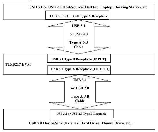
Figure 1. TUSB217 Functional System Level Block Diagram
