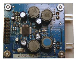
Figure 1. TAS5708(TAS5710)EVM Printed-Circuit Board
