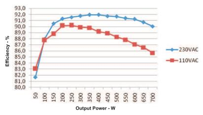
Figure 6. Efficiency at 50V Rail Voltage
