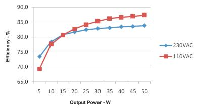
Figure 7. Efficiency at 25V Rail Voltage
