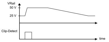
Figure 2. Correlation Between Rail Voltage and Clip-Detect Signal
