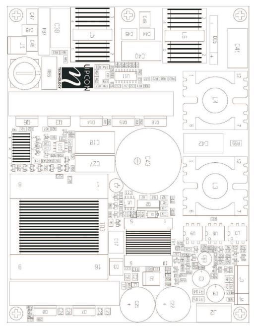
**Figure 17. Component Placement**
