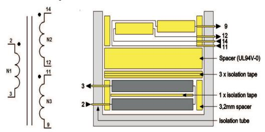
**Figure 4. Transformer Construction**
