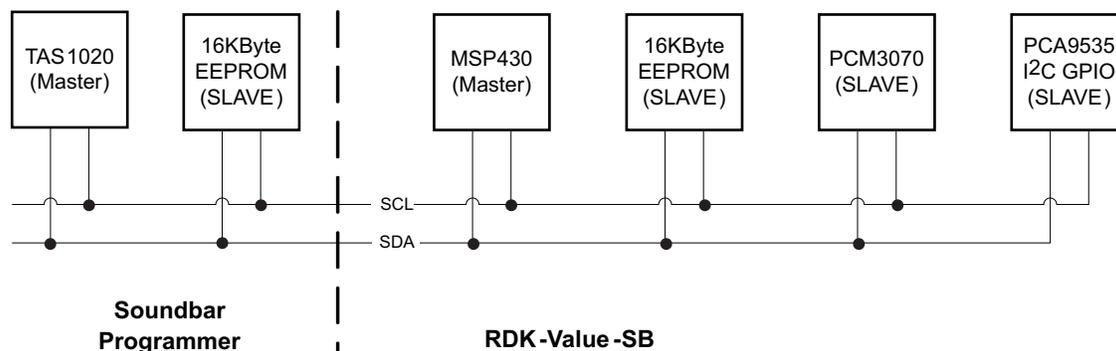
In a typical final product, the Soundbar Programmer board is not attached. It is only used for development, and potentially, production line programming. The power supply on the RDK-Value-SB actually powers the TAS1020 streaming controller on the RDK-Value-SB. As such, the 3V3 regulator on the soundbar may dissipate a little more heat in development than in final use.
