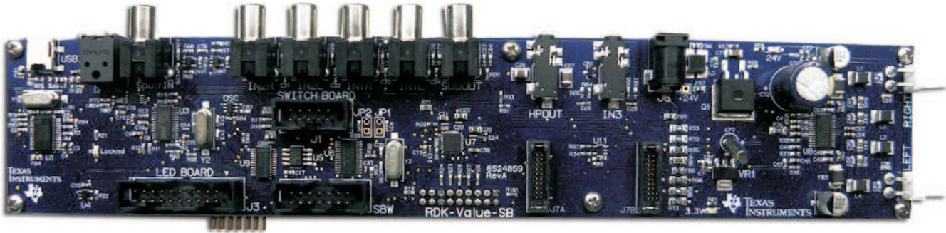
This document introduces the Value Soundbar Reference Design Kit from Texas Instruments. This reference design is the first of many that will span the complete market, from entry-level soundbars (ADC + I<sup>2</sup>S input amplifier) through to high-performance, multichannel soundbar reference designs incorporating Dolby AC-3 decoders, etc.
