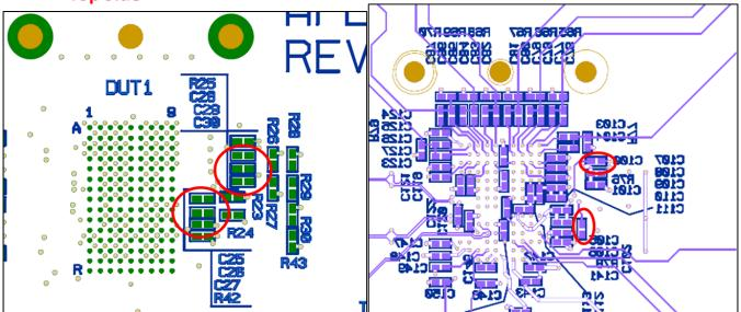
Figure 22. Relevant Capacitors for CW Mode, Top and Bottom Side
