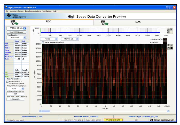
Figure 14. MSB and LSB Mismatch Raw Data for Sine Test Mode
