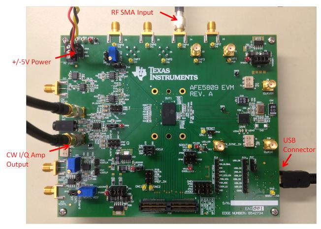
Figure 19. Setup for CW Mode
