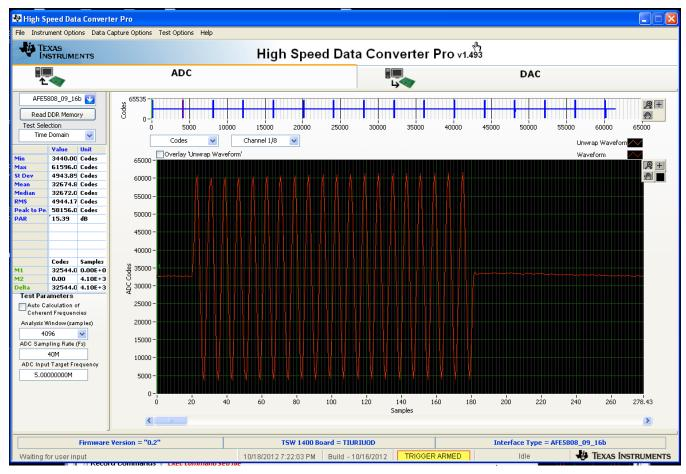
Figure 11. Analog Sine Burst with 20 Cycles at 10 MHz
