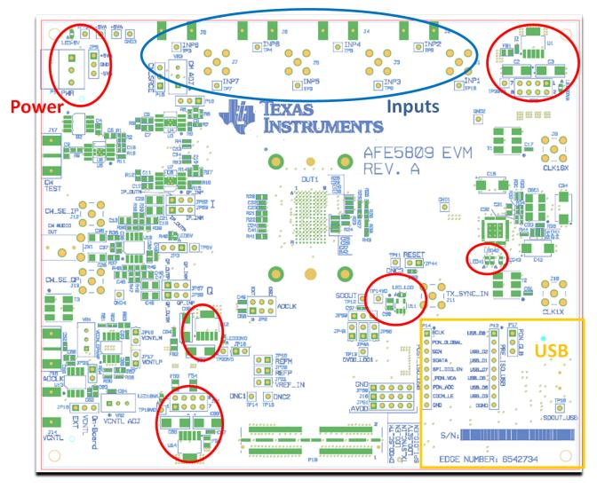
Figure 26. I/O, PWR, and USB Connector
