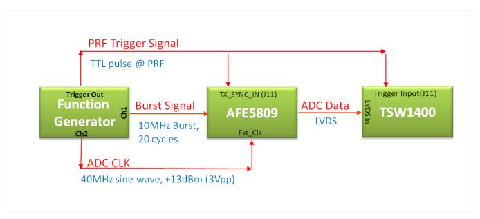
Figure 10. Hardware Setup for Demodulation Mode Capture
