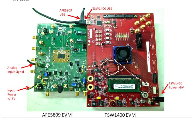
Figure 2. Default HW Setup With Connection Between TSW1400EVM and AFE5809
