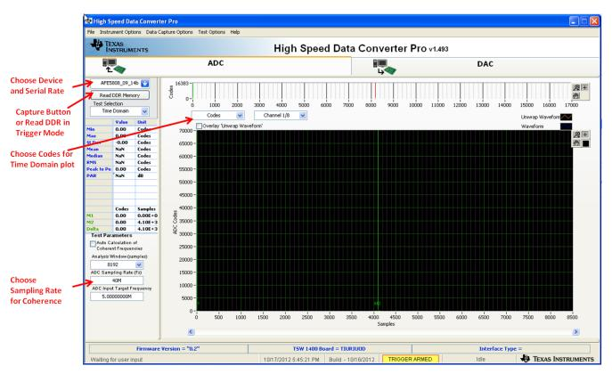
Figure 7. TSW1400 GUI Configuration
