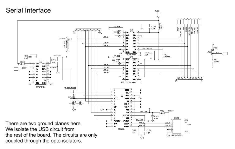
Figure 45. Schematic (Sheet 9 of 10)
