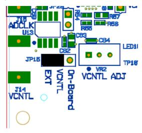
Figure 25. External Vcntl Configuration
