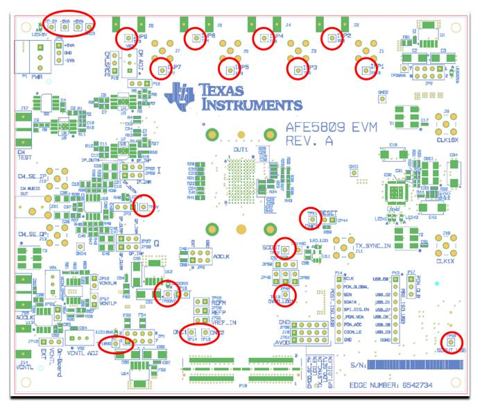
Figure 30. AFE5809EVM Test Point Locations
