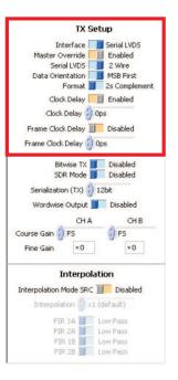
The data coming from the TSW1400 is edge aligned while the AFE722x expects the serial LVDS data to arrive edge centered. Here the programmable clock delay can be used to delay the edge-aligned clock closer towards the center of the data.
