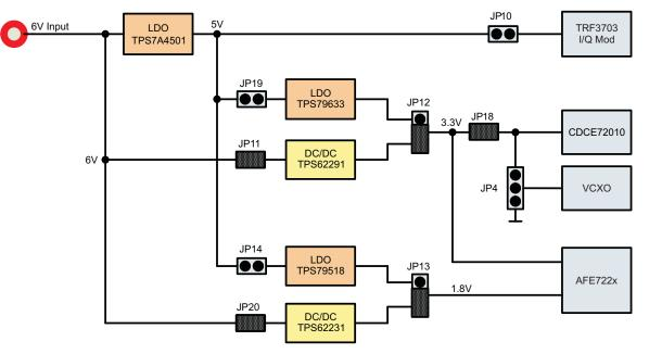
Figure 9. Power Supply Jumper Settings
