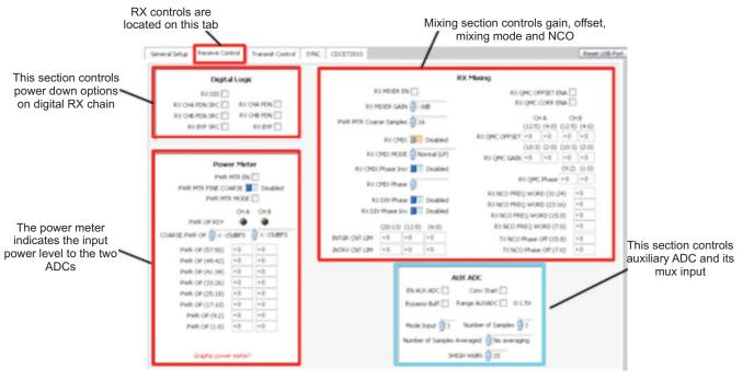
Figure 11. Receive Control Tab in RX Setup
