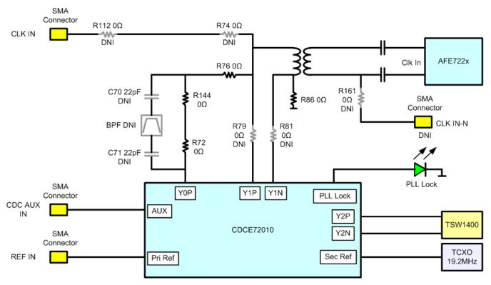
Figure 10. Configuration of Clock Output in CDCE72010
