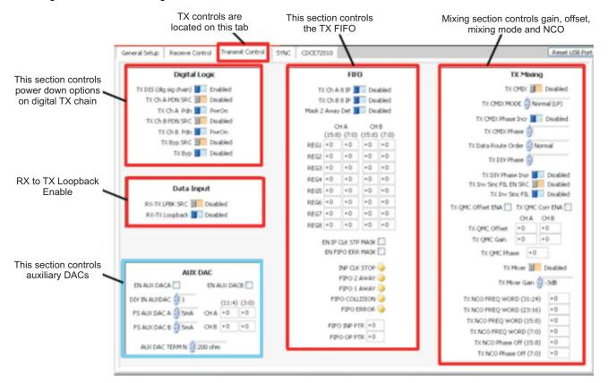
Figure 13. Transmit Control Tab in TX Setup
