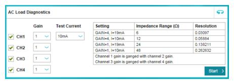
Figure 16. AC Load Diagnostics Section
