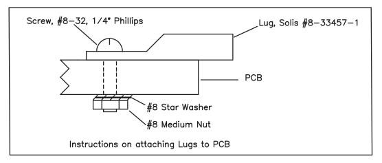
Figure 4. Lug Assembly Detail
