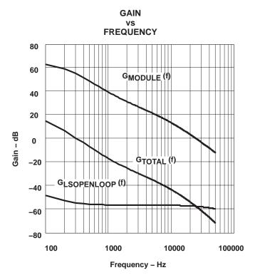
Figure 13. Load Share Open Loop Gain Frequency Response
