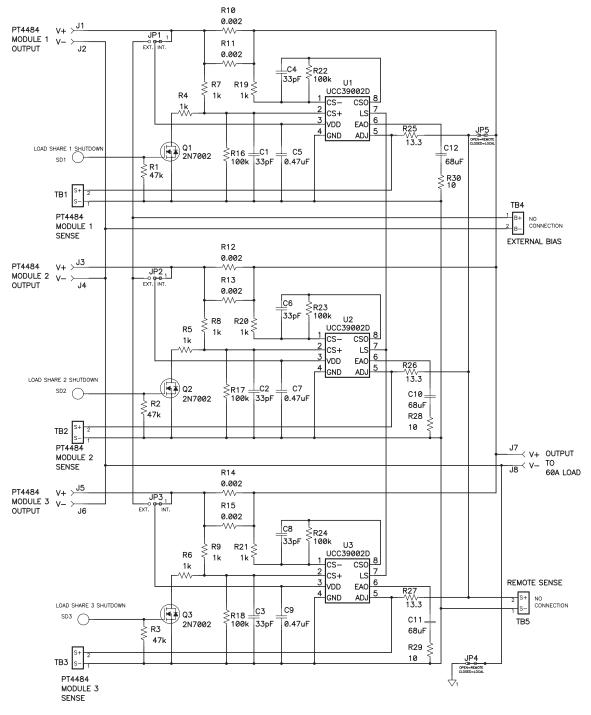
Figure 14. Schematic of Three Paralleled PT4484 Modules
