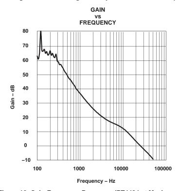
Figure 10. Gain-Frequency Response (PT4484 at Maximum Load)
