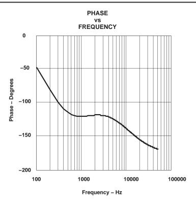
Figure 12. Phase-Frequency Mathematical Approximation of the PT4484 Module
