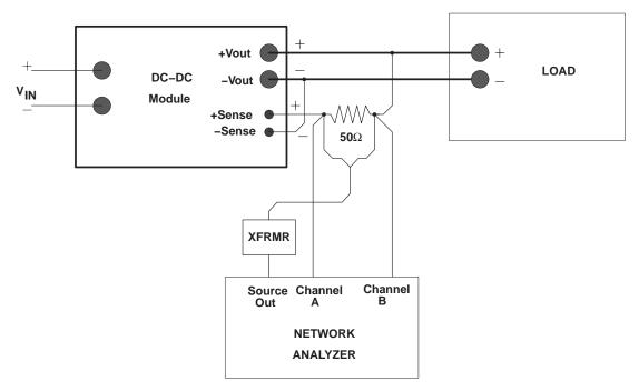
Figure 2. Measuring the Unity Gain Crossover Frequency
