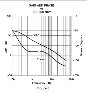
Figure 3 shows an example of the gain and phase frequency response measurement of a power module.
