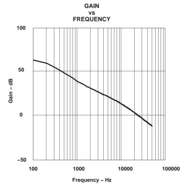
Figure 11. Gain-Frequency Mathematical Approximation of the PT4484 Module
