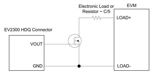
Figure 12. Load and Switch
