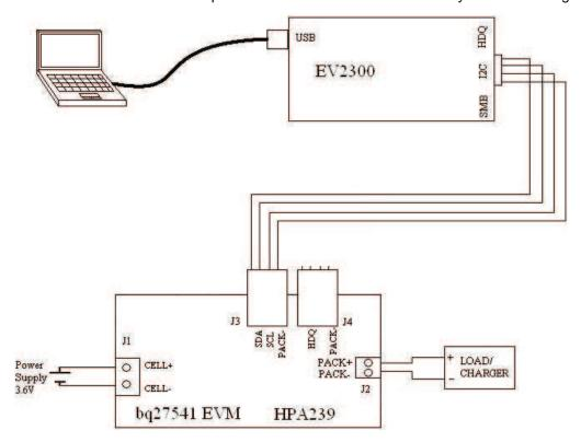
Figure 6. bq27541 Circuit Module Connection to Cell and System Load/Charger
