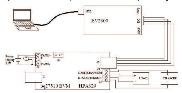
Figure 6. bq27510 Circuit Module Connection to Cell and System Load/Charger
