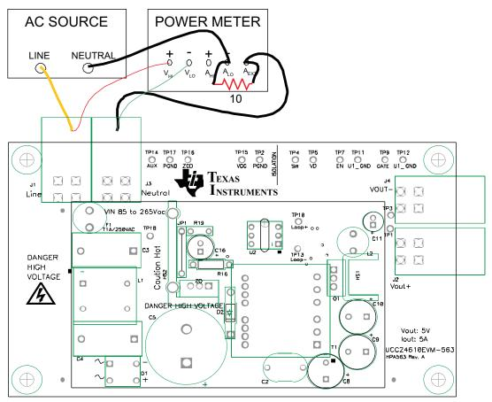
Figure 2. Recommended Test Set Up Without a Load.
