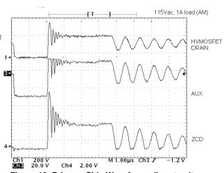
Figure 13. Primary-Side Waveforms (Input voltage = 115-V<sub>AC</sub>, 1-A load, Amplitude Modulation Mode.)
