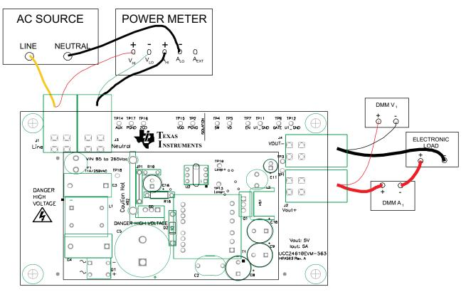
Figure 3. Recommended Test Set Up With a Load.
