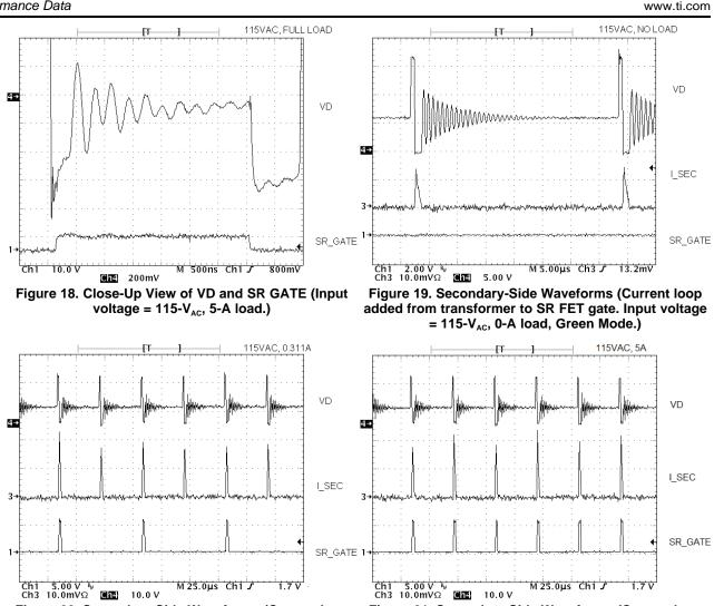
Figure 20. Secondary-Side Waveforms (Current loop added between transformer and SR FET gate. Low power mode. Input voltage = 115-V<sub>AC</sub>, 0.311-A load.)
