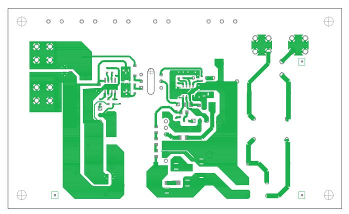
Figure 33. Bottom Layer Copper
