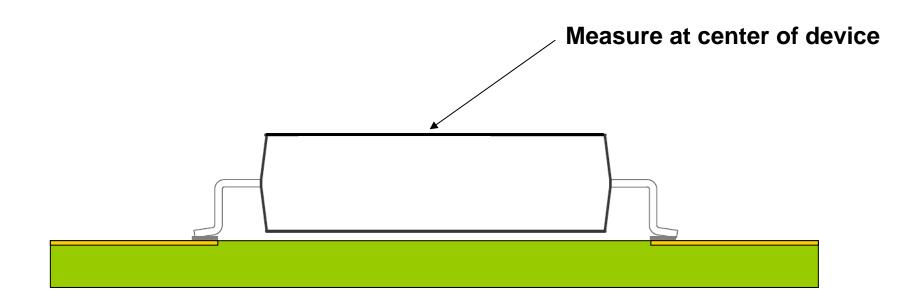
Measure device case temperature  $\mathrm{T}_{\mathrm{case}}$  using IR camera or thermocouple.
