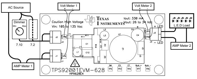
Figure 2. Recommended Test Set Up
