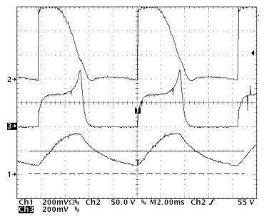
Figure 25. LED Current vs. Triac Conduction Time (Ch1- LED current Ch2- bulk voltage Ch3- U2-1 voltage waveform)
