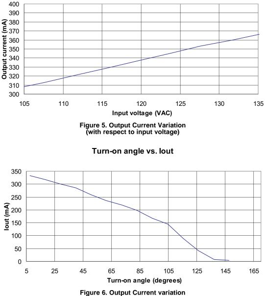
Input voltage vs. Output current
