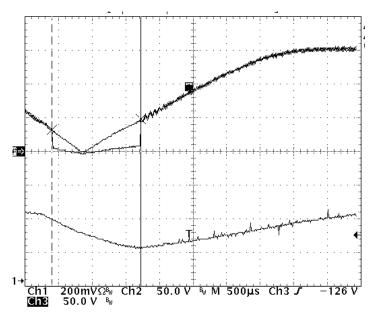
Figure 12. Dummy Load Conduction Time (Ch1- LED current Ch2- Q4 collector voltage Ch3- bulk voltage)
