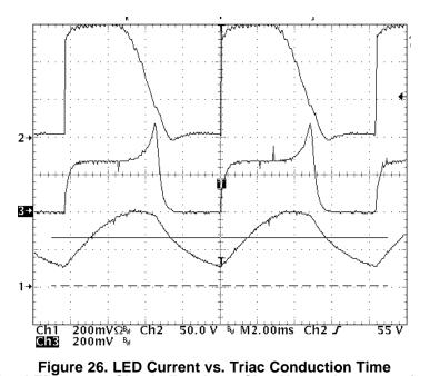
(Ch1- LED current Ch2- bulk voltage Ch3- U2-1 voltage waveform)
