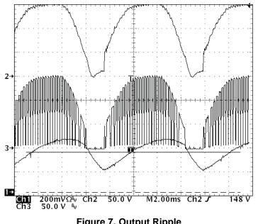
Figure 7. Output Ripple (Ch1-LED current Ch2- rectified line voltage Ch3- Q2 drain)
