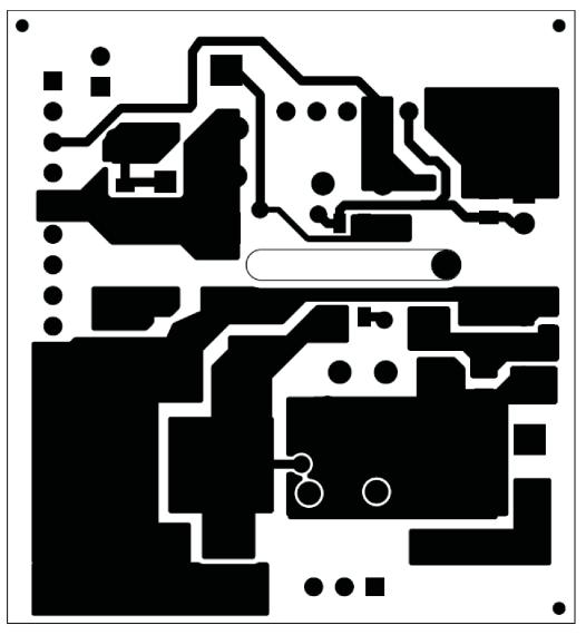
Figure 13. UCC27531EVM-184 Bottom Copper (top view)
