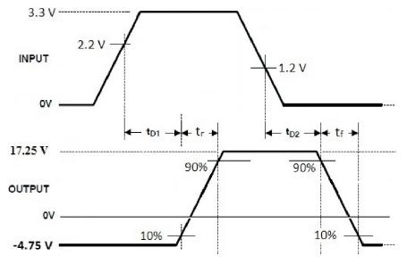
Figure 5. UCC27531EVM-184 Input vs. Output waveforms
