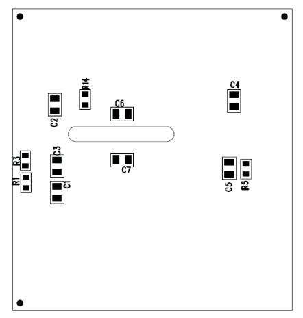
Figure 11. UCC27531EVM-184 Bottom Assembly Drawing (bottom view)
