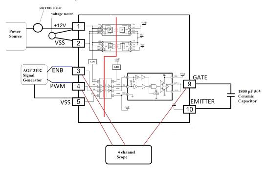
Figure 4. Recommended Test Setup
