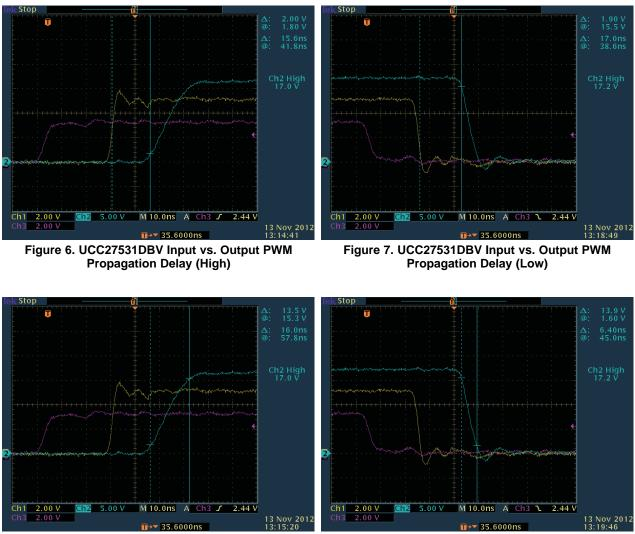
Figure 9. UCC27531DBV Input vs. Output PWM Fall Time
