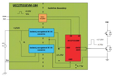
Figure 1. Low-Side Driver Configuration
