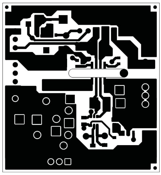
Figure 12. UCC27531EVM-184 Top Copper (top view)
