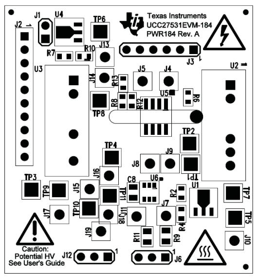
Figure 10. UCC27531EVM-184 Top Layer Assembly Drawing (top view)
