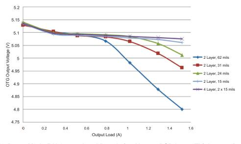
Figure 1. OTG Boost Mode 5-V Output Load Regulation Versus PCB Layer Thickness - Default Setting
