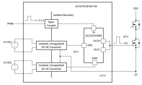
Figure 1. Low-Side Driver Configuration
