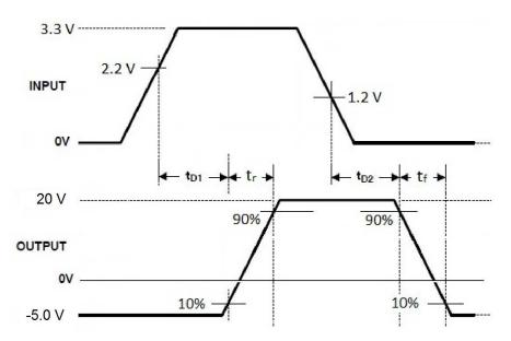
Figure 5. UCC27532EVM-538 Input vs. Output waveforms
