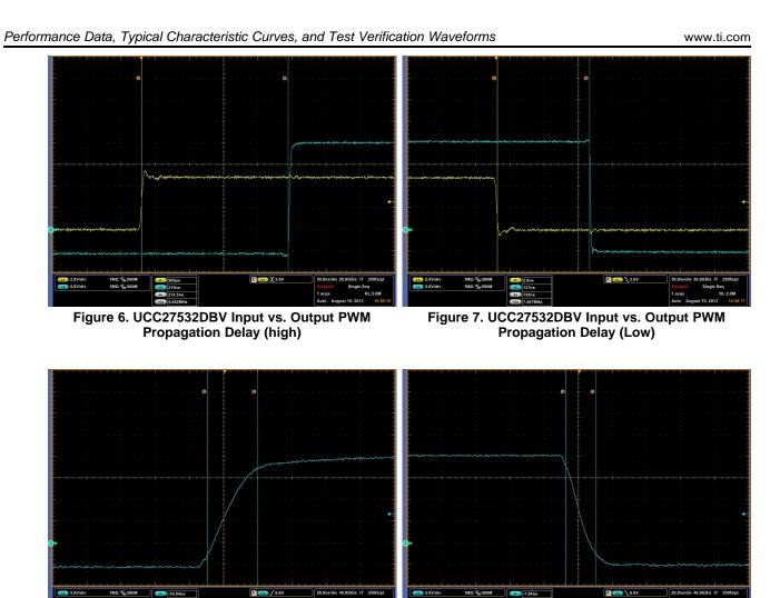
Figure 8. UCC27532DBV Input vs. Output PWM Rise F Time
