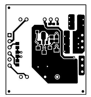
Figure 13. UCC27532EVM-538 Bottom Copper (top view)
