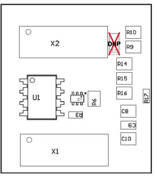
Figure 10. UCC27532EVM-538 Top Layer Assembly Drawing (top view)
