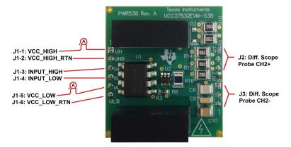
Figure 4. Recommended Test Setup
