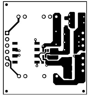
Figure 12. UCC27532EVM-538 Top Copper (top view)
