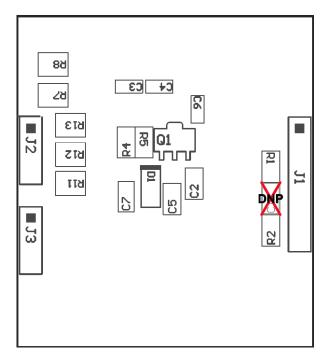
Figure 11. UCC27532EVM-538 Top Layer Assembly Drawing (top view)
