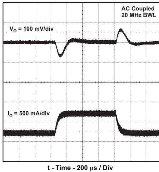
Figure 8. TPS5410 5 V Output Transient Response
