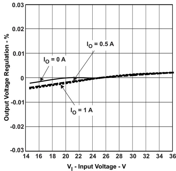
Figure 6. TPS5410 5 V Output Line Regulation
