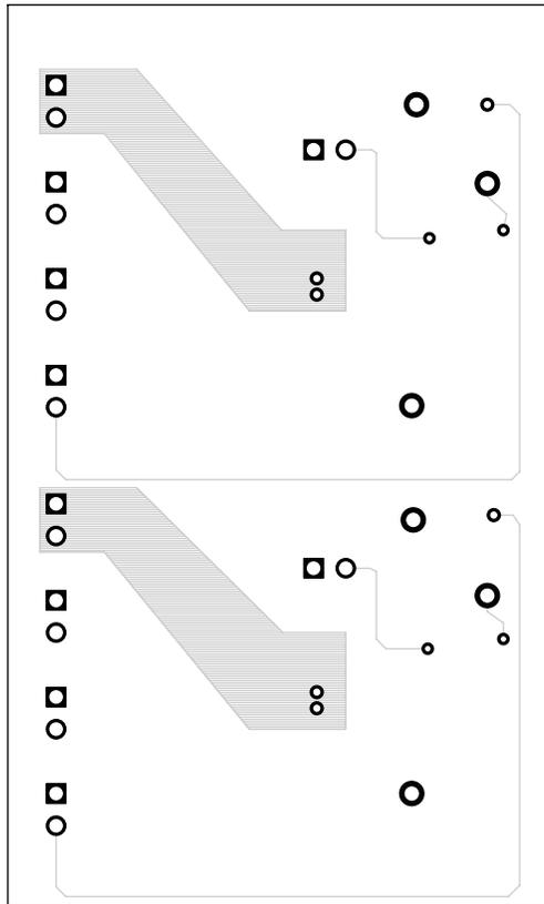
**Figure 18. Bottom-Side Layout (Looking From Top Side)**
