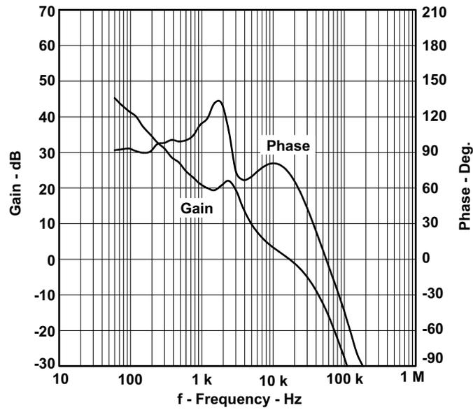
Figure 10. TPS5410 5 V Output Loop Response
