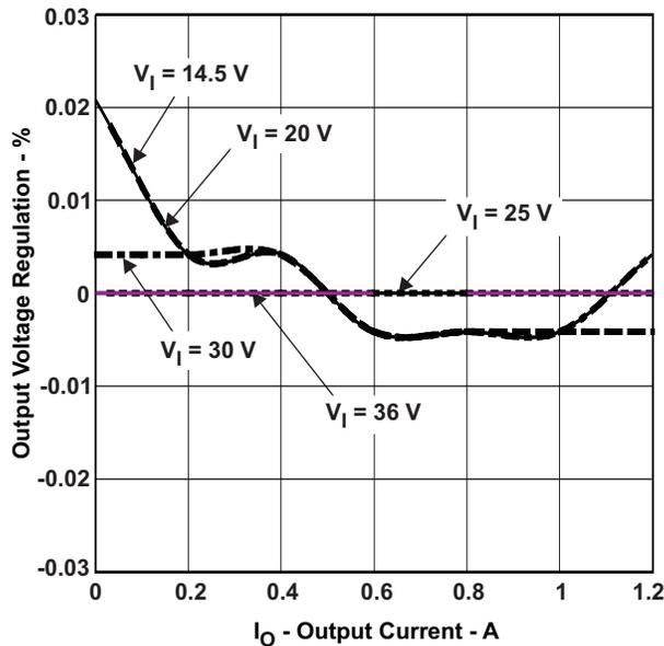
Figure 3. TPS5410 12 V Output Load Regulation
