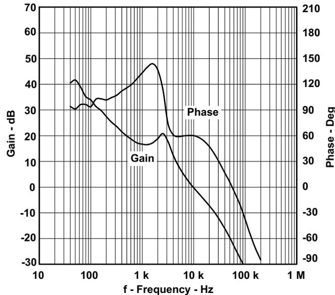
Figure 9. TPS5410 12 V Output Loop Response
