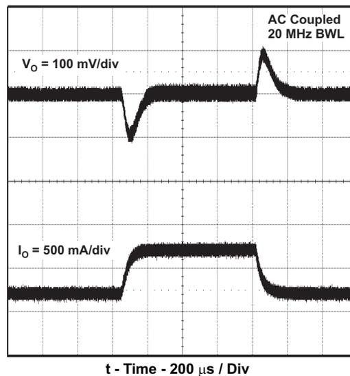
Figure 7. TPS5410 12 V Output Transient Response
