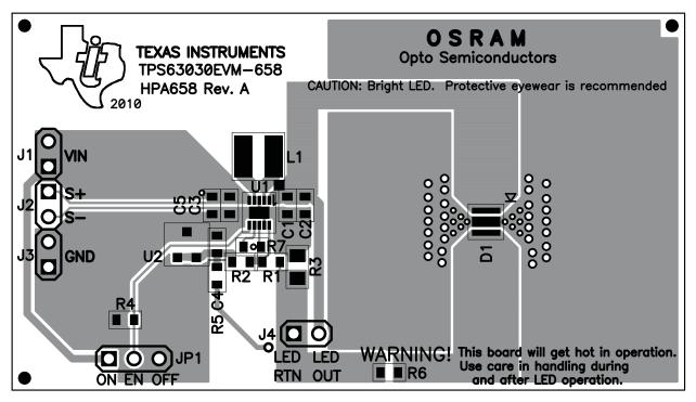
Figure 2. Assembly Layer Including Silk Screen
