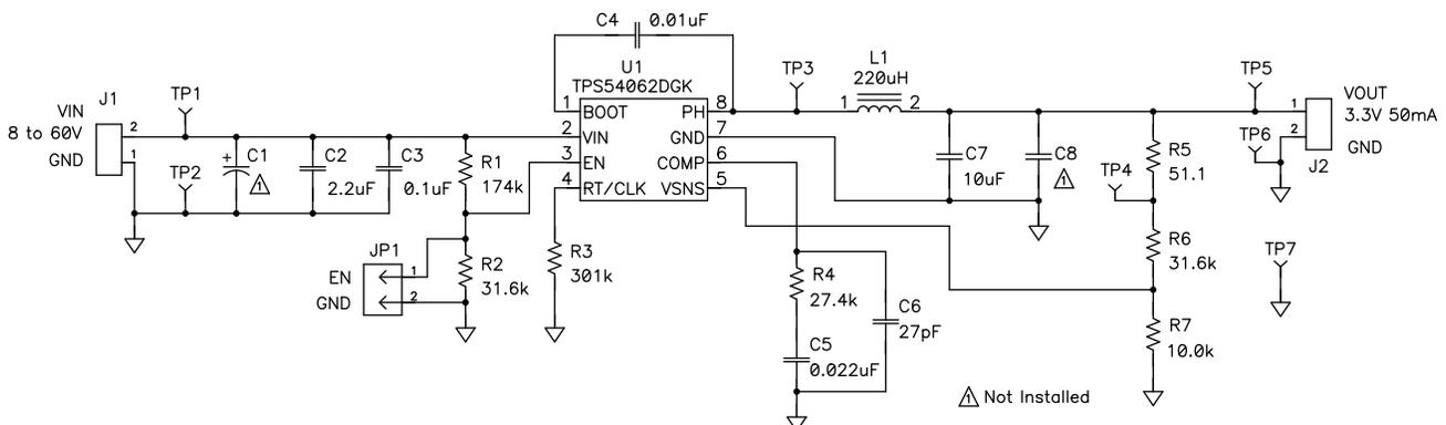
Figure 21. TPS54062EVM-695 Schematic
