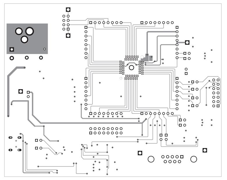
Figure 5. Layer-2 Routing
