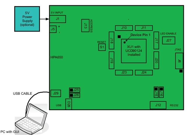
Figure 1. Typical Test Setup
