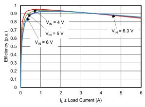
Figure 1. TPS50601SPEVM Efficiency
