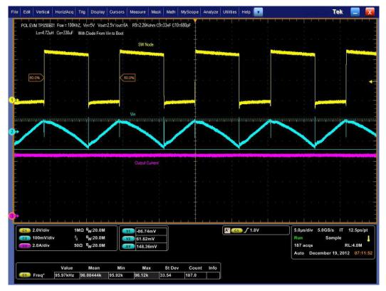
Figure 11. TPS50601SPEVM Input Ripple
