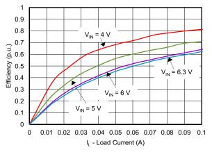
Figure 2. TPS50601SPEVM Low-Current Efficiency
