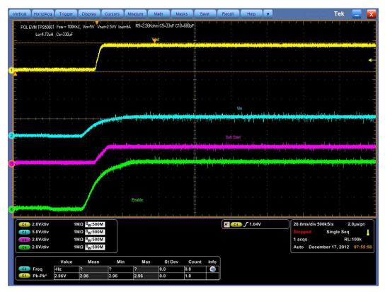
Figure 14. TPS50601SPEVM Start-Up Relative to V<sub>IN</sub>
