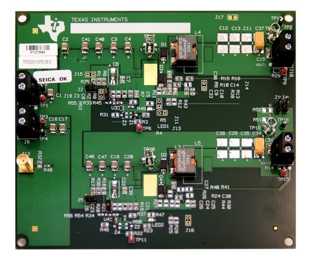
Figure 20. TPS50601SPEVM Bottom-Side Assembly
