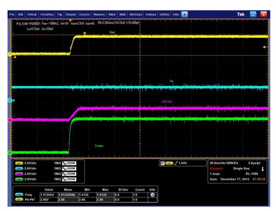
Figure 15. TPS50601SPEVM Start-up Relative to Enable
