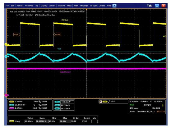
Figure 10. TPS50601SPEVM Output Ripple
