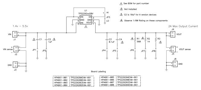
Figure 4. TPS2292xxEVM-661 Schematic
