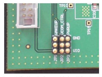
Figure 6. JP1, JP2, and JP3 Must Be Removed Before Using the GUI GPIO Control
