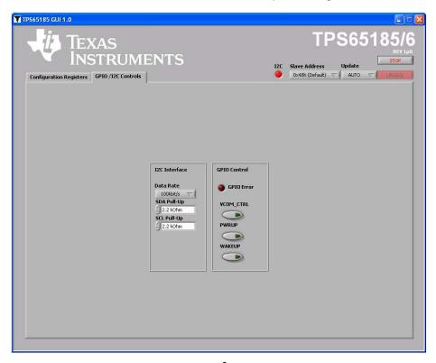
Figure 5. GPIO/I<sup>2</sup>C Control Tab
