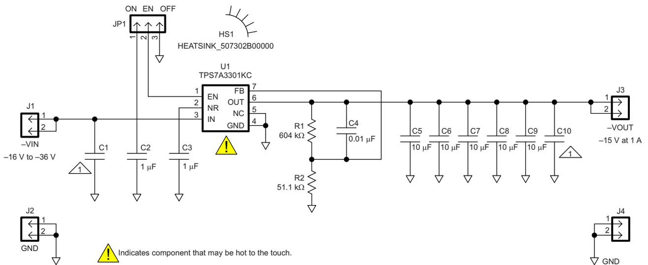
Figure 7. TPS7A3301EVM-061 Schematic
