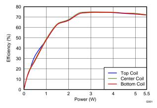
Figure 5. Efficiency Versus Power Across Each Coil, bq500410AEVM-085 Transmitter and bq51013AEVM-764 Receiver
