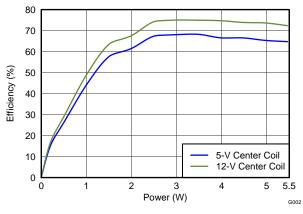
Figure 6. Efficiency Versus Power Center Coil 12-V Input Versus 5-V Input, bq500410-085 Transmitter and bq51013AEVM-764 Receiver
