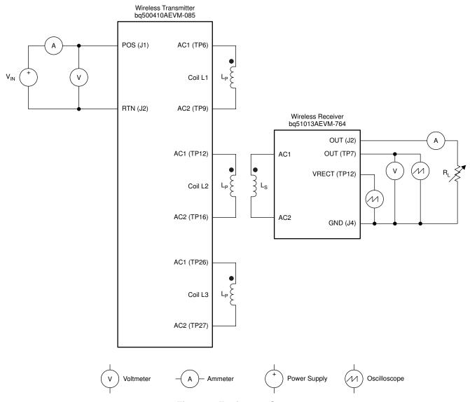
Figure 4. Equipment Setup
