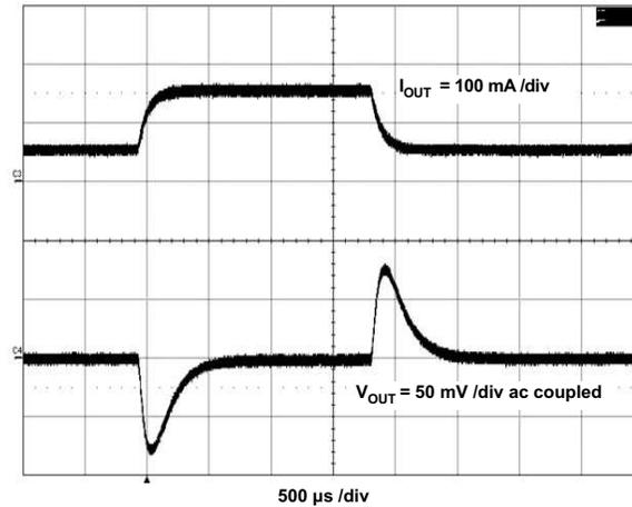
Figure 5. TPS54061EVM-142 Load Transient Response
