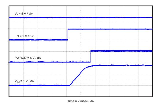
Figure 10. TPS54719EVM-152 Start-Up Relative to Enable
