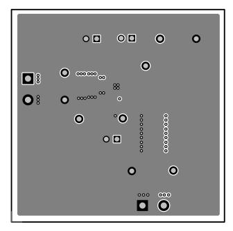
Figure 16. TPS54719EVM-152 Internal Layer 2 Layout
