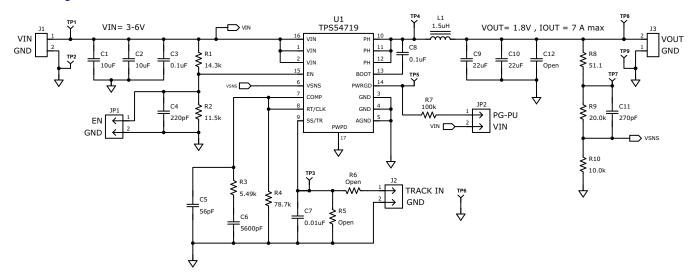
Figure 18. TPS54719EVM-152 Schematic
