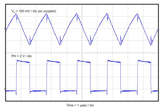
Figure 8. TPS54719EVM-152 Input Ripple
