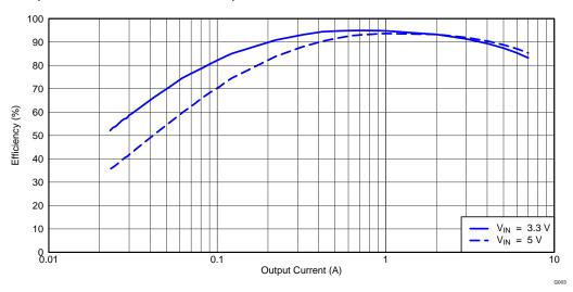
Figure 2. TPS54719EVM-152 Low Current Efficiency
