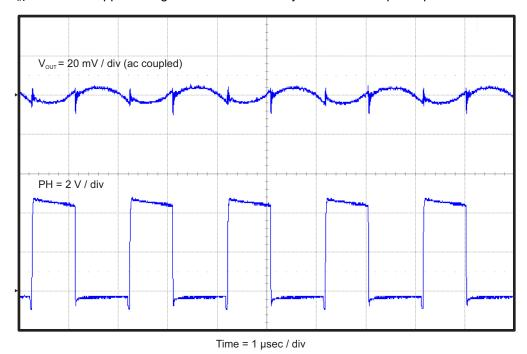
Figure 7. TPS54719EVM-152 Output Ripple
