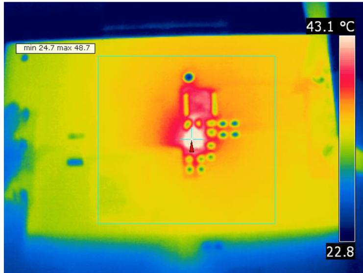
Figure 2. Thermal Performance ( $V_{IN} = 6\text{ V}$ , Load = 3 A)
