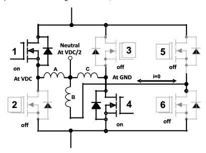
Figure 31. Motor Neutral Voltage During PWM On Period
