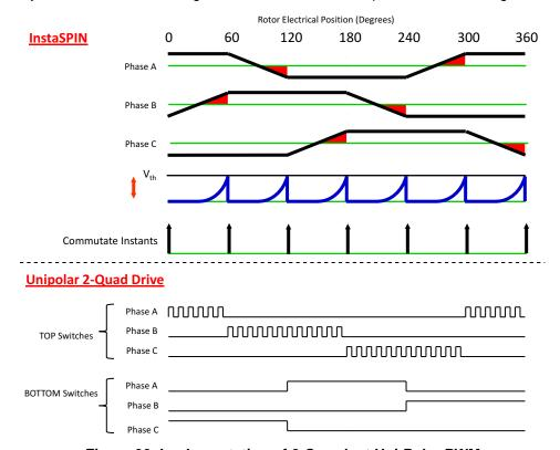
Figure 30. Implementation of 2-Quardent Uni-Polar PWM
