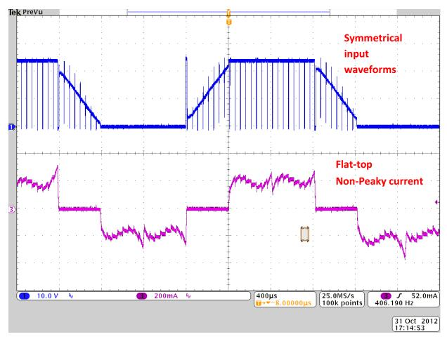
Figure 33. Typical Waveform for the OPTIMUM Flux Threshold
