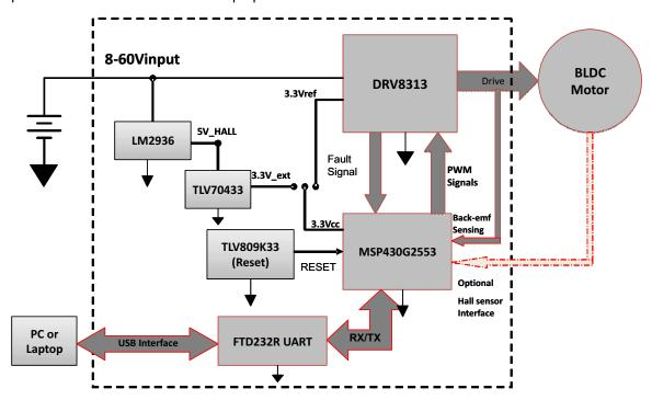
Figure 2. DRV8313EVM Hardware Block Diagram
