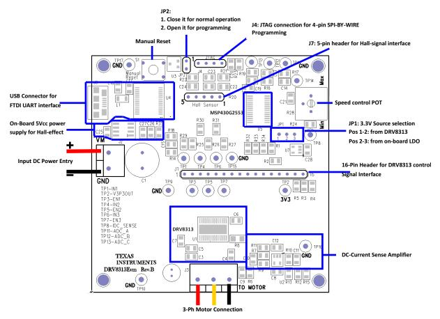
Figure 3. DRV8313EVM Macro Blocks and Jumper Setting
