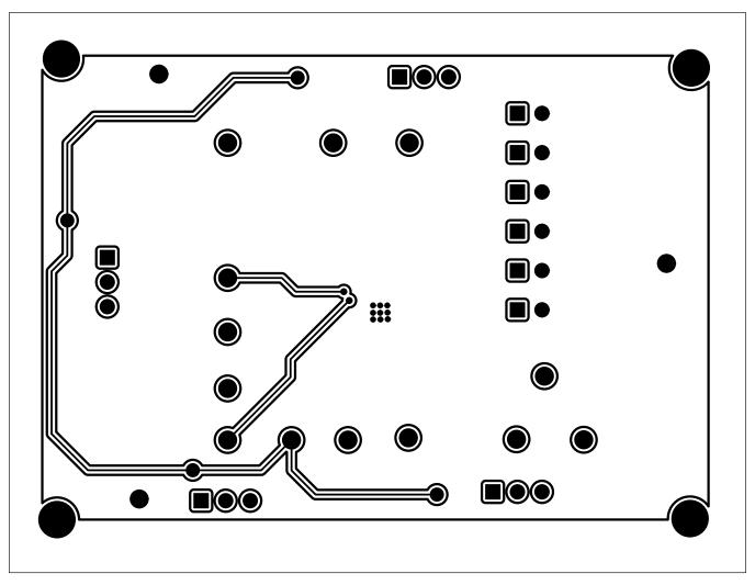
Figure 3. Bottom Layer Routing
