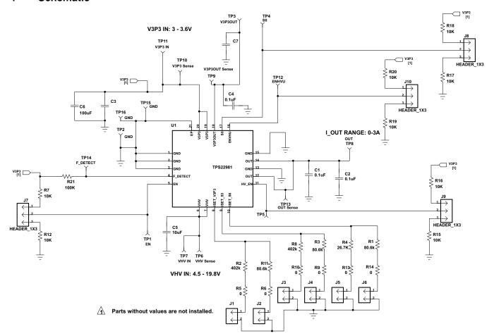
Figure 4. TPS22981EVM Schematic
