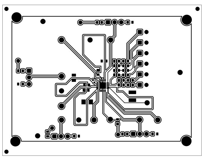
Figure 2. Top Layer Routing
