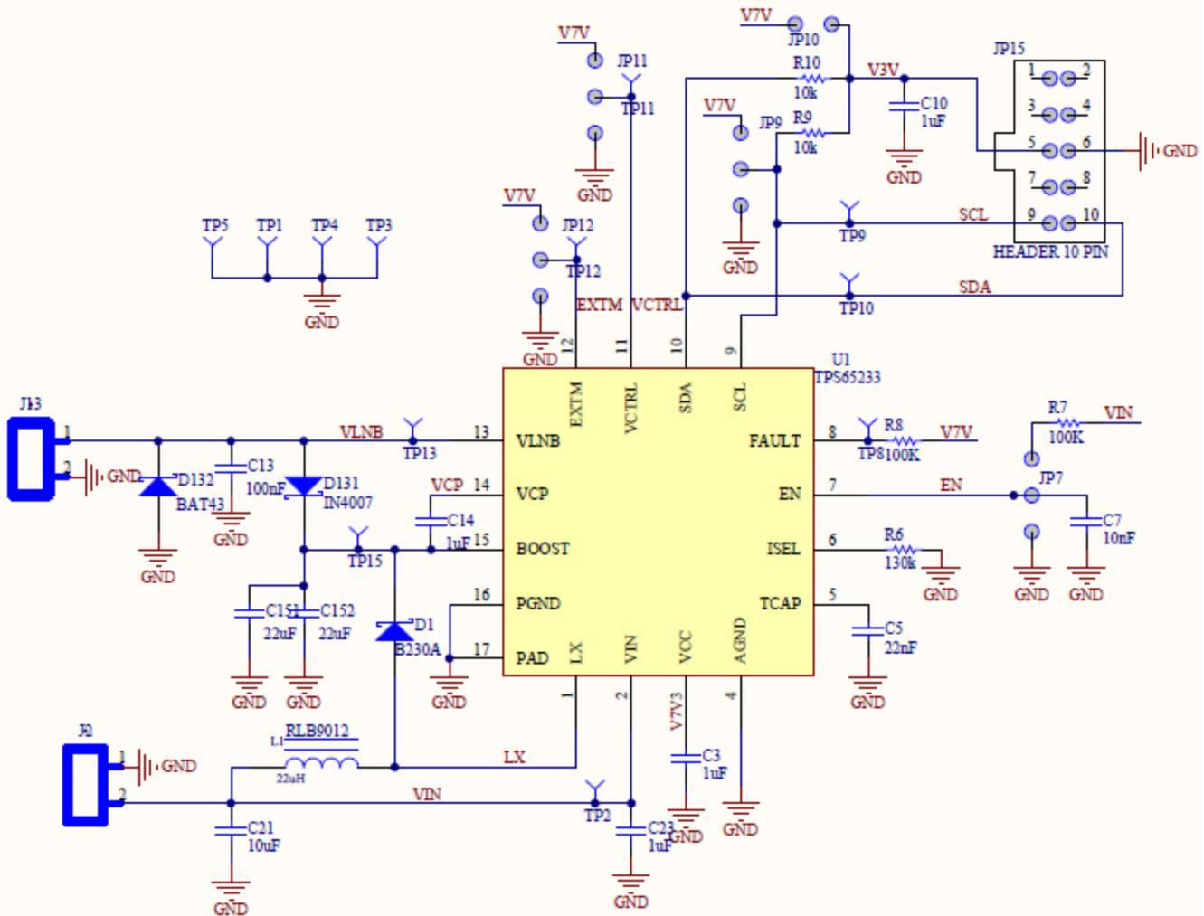
Figure 17. TPS65233EVM Schematic
