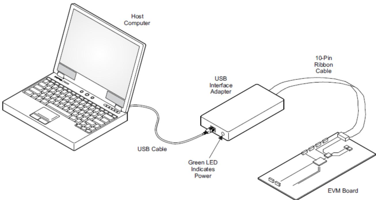
**Figure 5. USB Interface Adapter Quick Connection Diagram**
