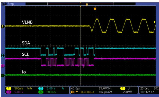
Figure 15. 22-kHz Tone Controlled by I<sup>2</sup>C,  $V_{IN} = 12\text{ V}$ ,  $V_{LNB} = 13.4\text{ V}$ ,  $I_o = 0\text{ A}$
