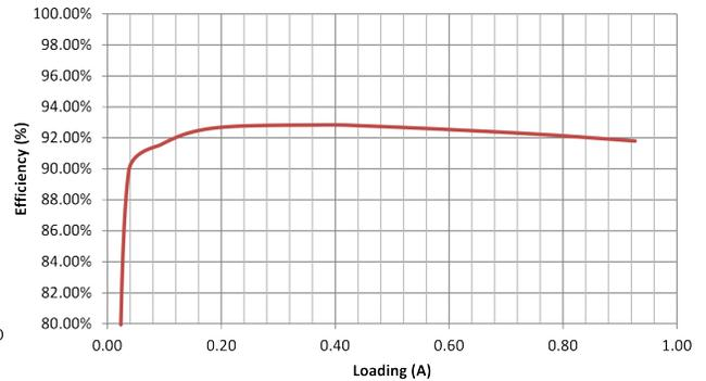
Figure 8. Efficiency,  $V_{IN} = 12\text{ V}$ ,  $VLNB = 18.6\text{ V}$
