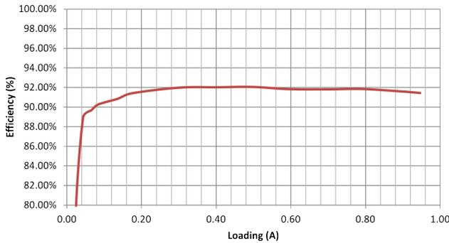
Figure 7. Efficiency,  $V_{IN} = 12\text{ V}$ ,  $VLNB = 13.5\text{ V}$
