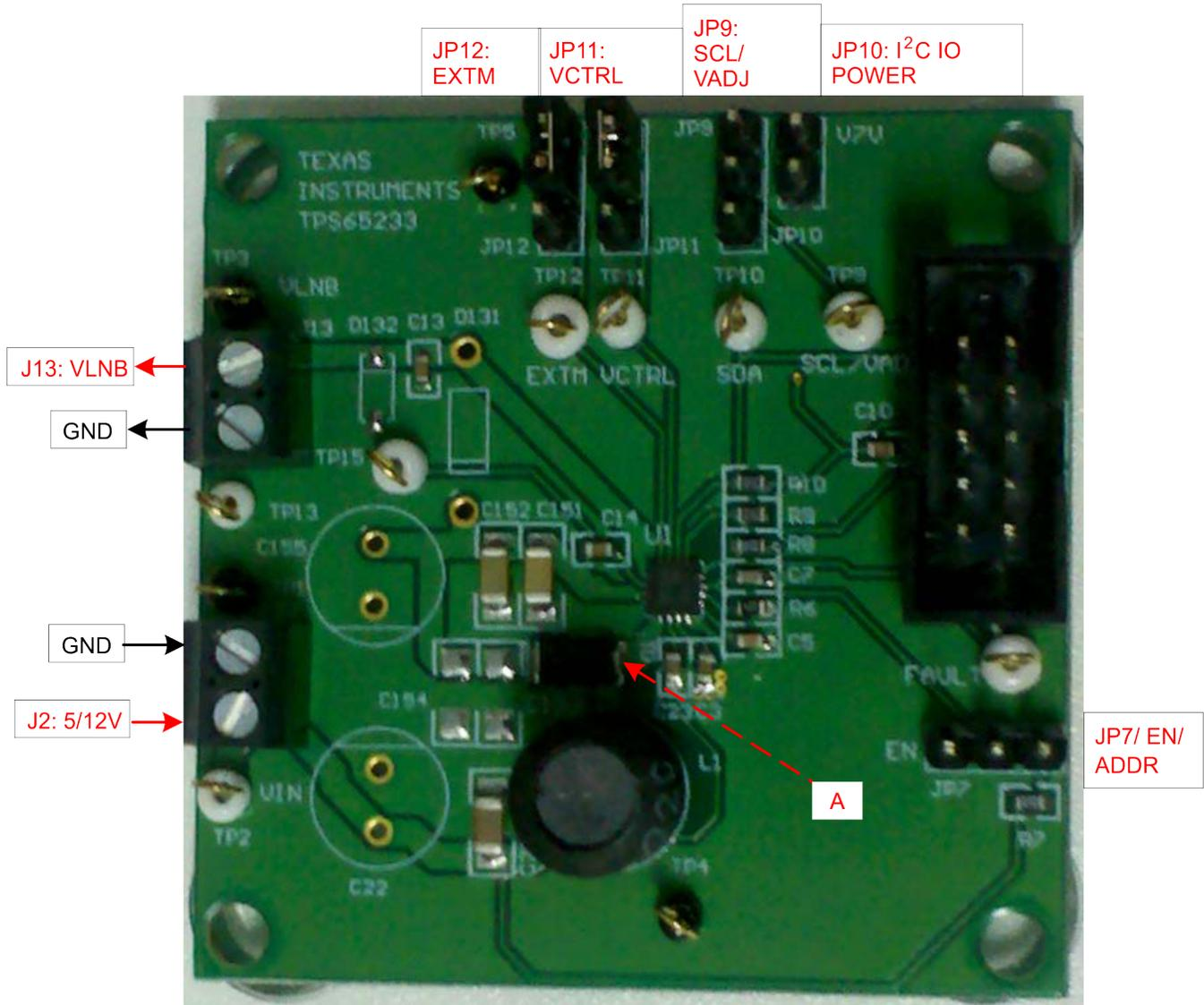
Figure 4. Headers Description and Jumper Placement
