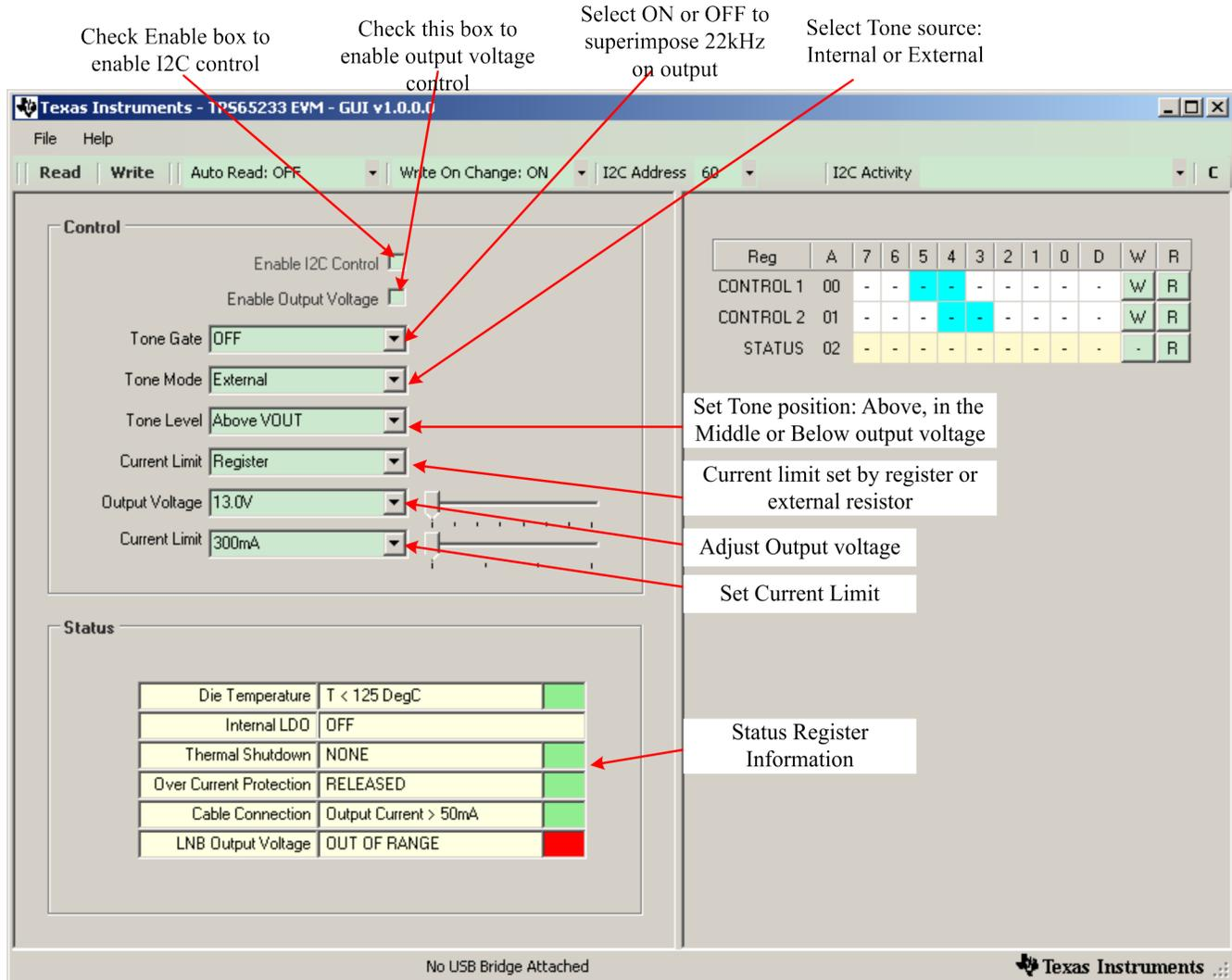
**Figure 6. Screen Capture of TPS65233 Software GUI Interface**
