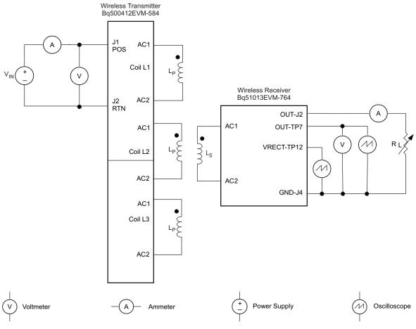
Figure 3. Equipment Setup
