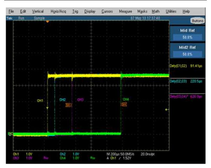
Figure 33. Programmable Turn on Delay Time
