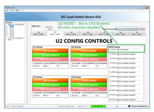
Figure 10. Set U2 Mode1 Register to CH2 Enabled
