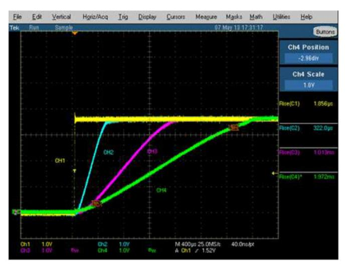
Figure 32. Programmable Slew Rate Control
