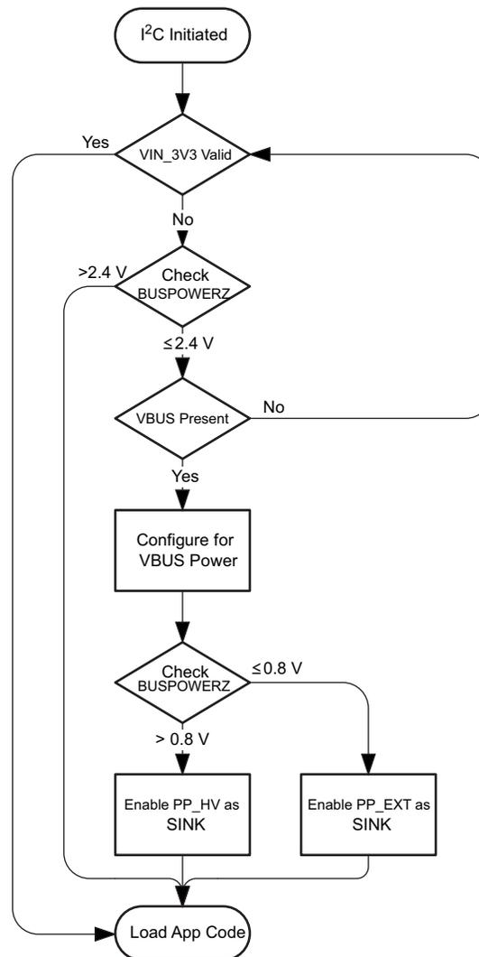
**Figure 3-3. Dead-Battery Process**
