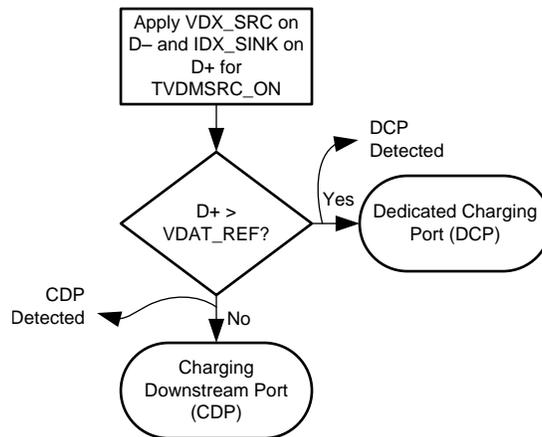
Figure 12-4. Secondary Detection
