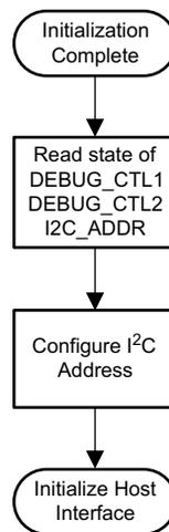
**Figure 3-2. I<sup>2</sup>C Address Configuration**
