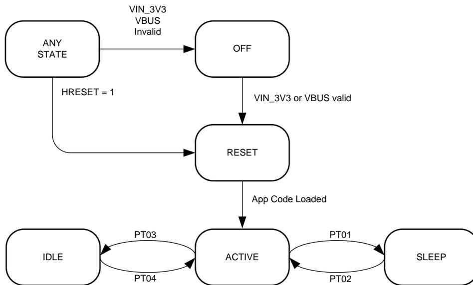
**Figure 5-1. Power State Diagram**
