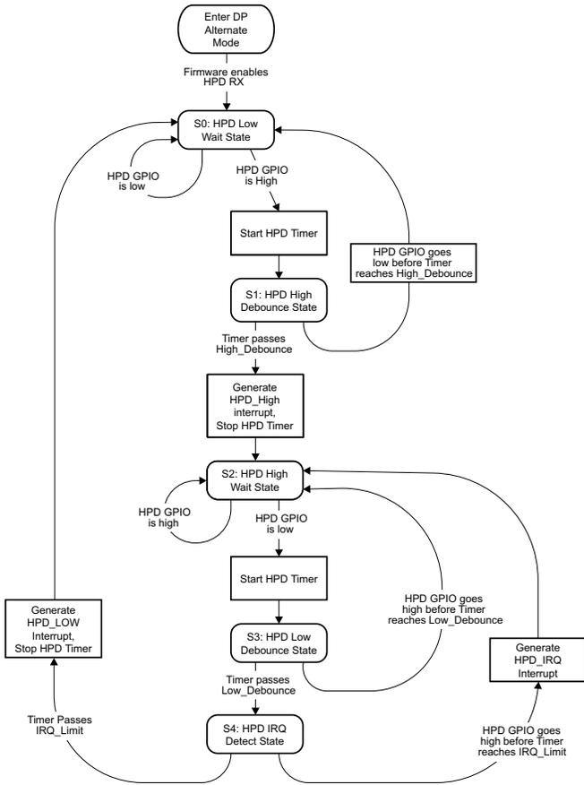
Figure 10-1. DisplayPort Sink-Side Hardware Flow (HPD RX)
