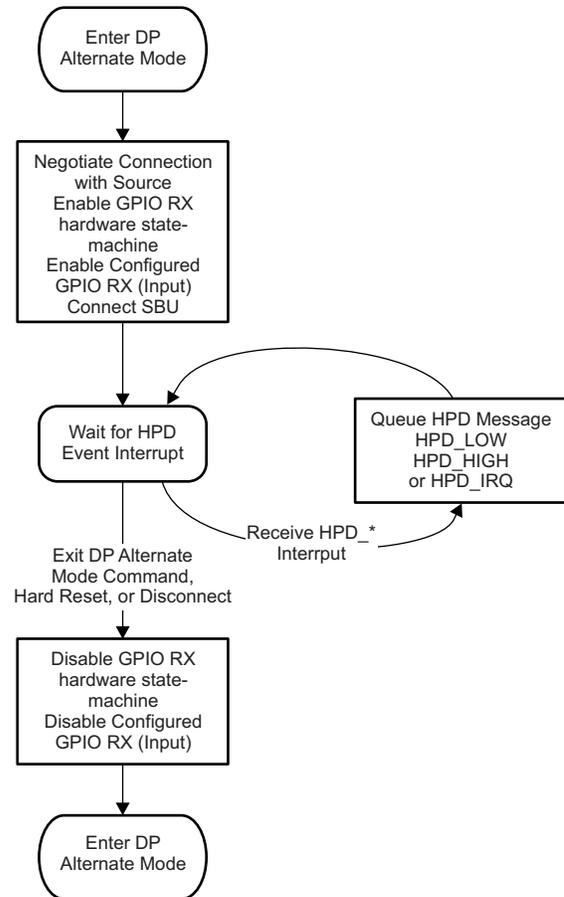
Figure 10-2. DisplayPort Sink-Side Firmware Flow (HPD RX)
